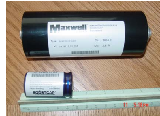
Above, 2700F BoostCAP & New D-Cell BoostCAP. Below, D-Cell 15V 58 F module
